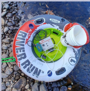
FOCs' eDNA raft and pump to take samples.
